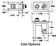
P - 3/4" Female Pipe Thread C - 3/4" Copper Sweat Fitting EP - Union Elbow with 3/4" Male Pipe Thread
